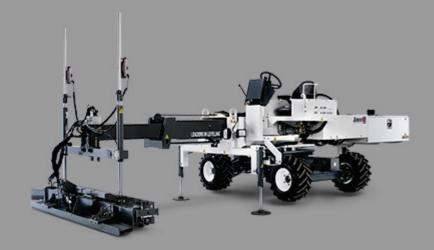
The S-15m Laser Screed concrete leveling machine screeds 15m 2 (160 sf) per pass with a 6m (20') telescopic boom reaching out over the concrete. The powerful hydraulic elevation cylinders control the plow and auger to maintain grade so you can get a much smoother surface vs. other methods, even with very low slump concrete!
