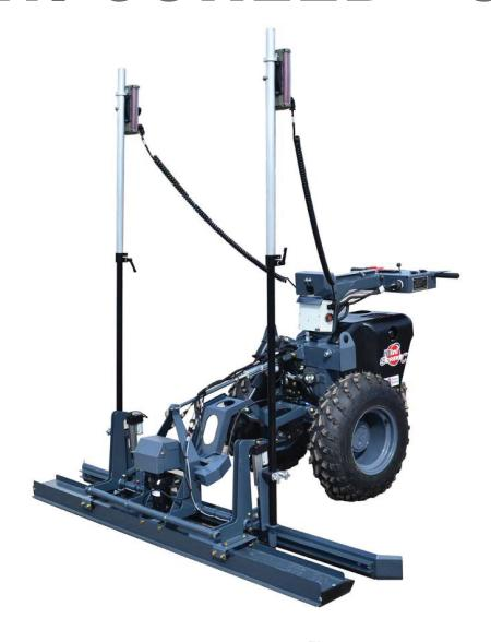
Get superior productivity and flatness with the Mini Screed  $^{\mathsf{TM}}$  C. Designed for small commercial, upper deck, and residential projects — the Mini Screed  $^{\mathsf{TM}}$  C provides you and your customers with high quality, professionally produced floors at a fraction of the cost of conventional methods. With laser-controlled accuracy, this machine will screed to higher tolerances than traditional methods and works well with cement mixes of varying slumps.
