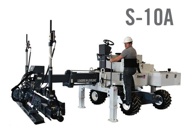
With operator conveniences unmatched in the industry, the S-10A was engineered for productivity and convenience. Despite its compact size, the S-10A is highly productive, screeding 200 square feet per pass thanks to its 20' / 6 m telescopic boom and a patented, fully-automated, self-leveling, 10' screed head. Surprisingly light weight, the S-10A Laser Screed® model can be easily transported.
