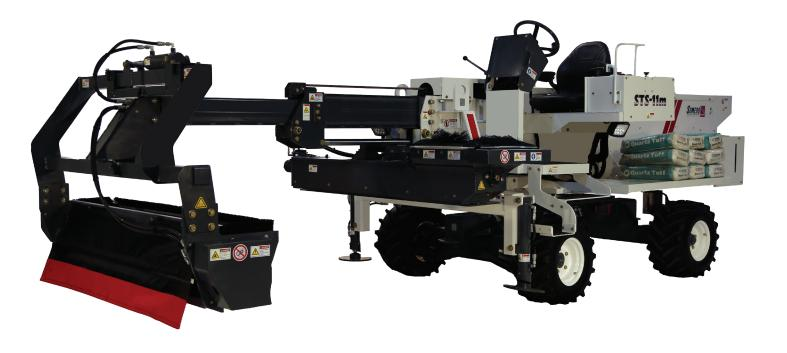
Disperse a wide variety of shake-on toppings with the **STS-11M** Topping Spreader. Its uniquely versatile design features a low dust loading technology with Inlet Hopper brushes, storage for up to twenty 50-lb. / 22.7 kg bags, and a compact machine size for easier transporting. The STS-11M Topping Spreader provides spreading accuracy that allows you to distribute shake-on toppings from fine materials to trap rock.
